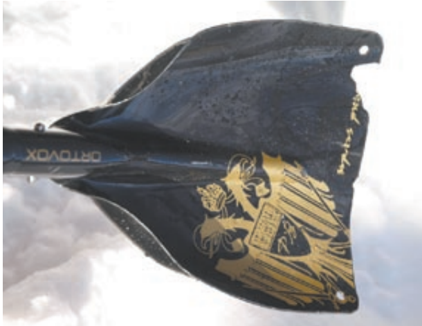
The Ortovox Alaska's weak material could not hold up to digging and chopping blocks.
