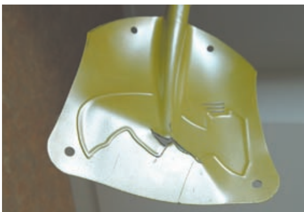
In short order, the Pieps blade was so severely deformed and cracked that the shovel could no longer function.
