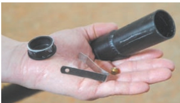
Stubai's locking bolts fell apart in different positions on several of the shovels tested, rendering them useless.
