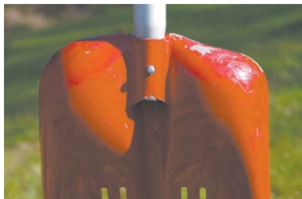
This G3 model held up well during testing, showing only minor deformation to the top edge that did not affect shovel performance.
