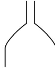
When the top of the blade slopes to the sides at an angle, the boot simply slides off preventing any energy from being transferred from the foot to the shovel. This wastes energy and causes the shoveler to become discouraged.
